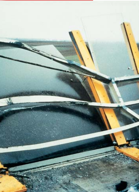
Top image: 240 kg ball dropped from a height of 6.4 m to an aged panel
